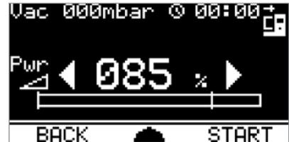
In the lower part of the Casting menu the currently specified power value is displayed as percentage in large numbers. You can change the default value anytime by turning the turning knob to the left or to the right.
