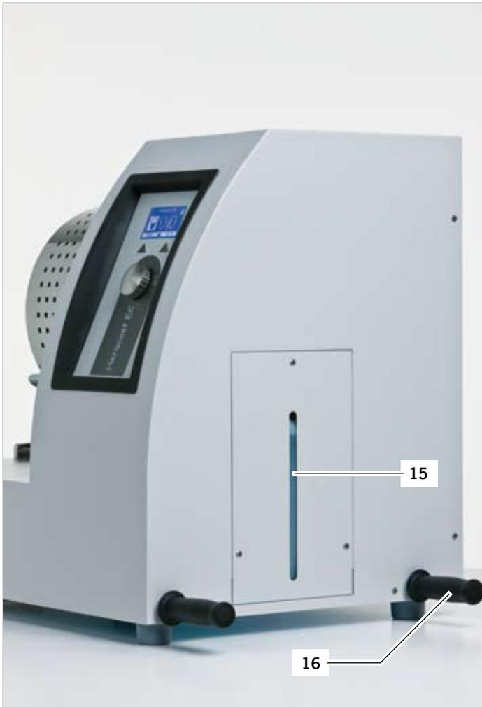
**15** Side trap door with viewing glass for cooling water level
