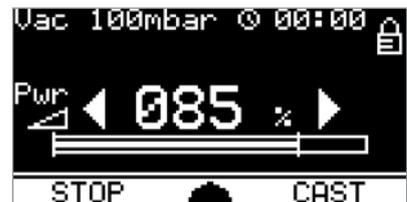
Push the “CAST” key to pivot the inductor coil and the casting ring immediately. Due to its own weight the melt will flow into the cavities of the casting mould. Simultaneously, compressed air is admitted to the chamber automatically (audible pressure surge) and the melt is pressed into the finest areas of the casting mould.
