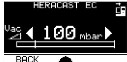
Push the “BACK” button to return to the previous menu. Push the turning knob to confirm the specified vacuum value.
