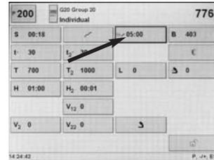
If a firing program with pre-vacuum is conducted, the vacuum pump is switched on at the end of the closing time (as soon as the furnace head is closed). Once the pre-vacuum time has elapsed, the heating phase begins. Upon the start of a program with an individually activated pre-vacuum (value between 1:00 and 5:00), the V1 value is ignored. The vacuum is maintained until V2 is reached. V2 must be higher than the stand-by temperature B.
