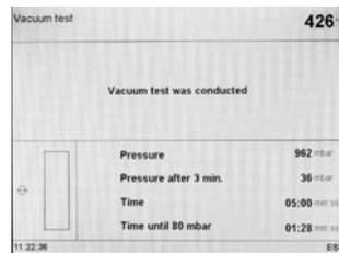
With this program, the vacuum performance of the furnace vacuum system can be automatically tested. For that purpose, the achieved (minimum) pressure in mbar is measured and indicated. If the pressure value is below 80 mbar (hPa), the vacuum performance of the system is adequate.
