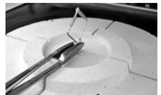
4. If necessary, use the furnace tongs to apply slight pressure to the center of the calibration base until the calibration sample clicks into place. Observe the corresponding markings.
