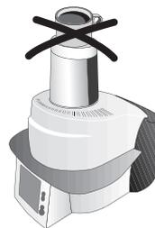
Foreign objects must not be placed on the air vents. Make sure that no liquids or other foreign objects enter the air vents, since this may result in an electrical shock.
