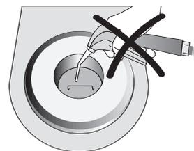
This product contains ceramic fibres and may release fibre dust. Do not use compressed air, or blow, on the furnace thus distributing the dust in the environment and observe the additional notes on page 11.
