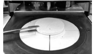
3. Carefully grip the upper part of the ATK 2 using the furnace tongs (Caution: Fracture risk of the ceramic) and insert it into the holes designated for this purpose until it snaps into place.
