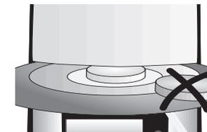
Firing trays must not be placed in the area surrounding the firing table, since this will obstruct the closing of the furnace head.
