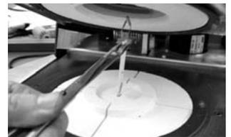
7. Replace the firing plate using the furnace tongs.
