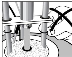
Mount the press drive cover (56) and fasten with screw.
