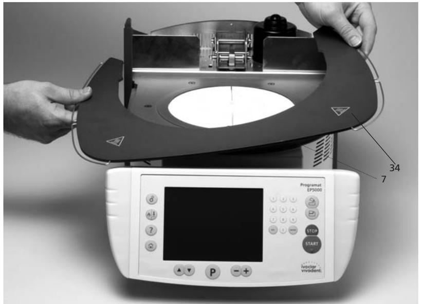
Secure the cooling tray L (34) with the two screws (35) including the silicone washer (47).
