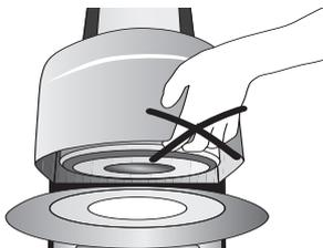
The furnace has an electric drive and must be operated by means of the electronic controls. Never open the furnace head by hand, since the mechanism will be damaged.
