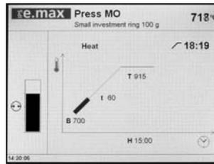
Operation screen during a press program in the Standard mode. Once the press procedure starts, an additional arrow indicates that the press plunger moves downwards. The entire time of the press cycle is displayed once and the path which the press plunger has already covered since the start of the press procedure in the selected measuring unit.
