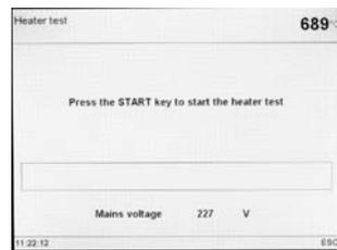
The quality of the heating muffle may be automatically checked by means of the heater test (duration: approximately 7 minutes). The heater test should only be conducted with the empty firing chamber, since an object in the chamber (e.g. firing tray) may influence the test result. Conduct the heater test
