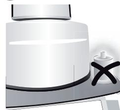
Do not cool the hot investment ring on the cooling tray. Use only the cooling grid for that purpose.
