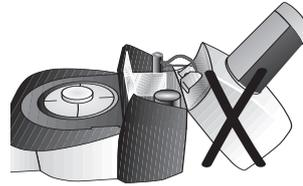
The furnace head should not be removed from the furnace base as long as the furnace head is connected by means of the heater cable.
