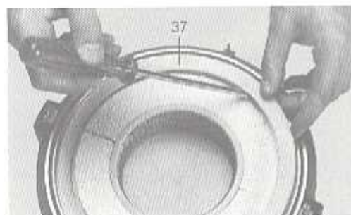
Fig. 18 Lever up and remove ring (37).
