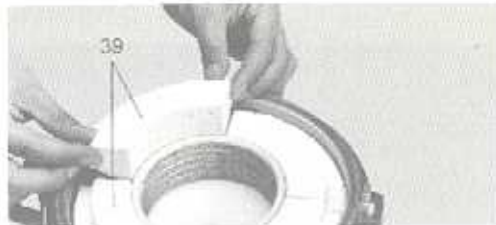
Fig. 20 Carefully remove the four spring ring segments (39).
