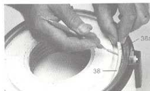
Fig. 19 Level out ends of insulation core (38a) with a spatula and gently pull out core (38) by hand.
